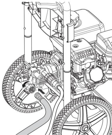
Completely uncoil garden hose or remove completely from reel to prevent kinks.
