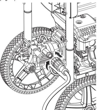
Completely uncoil and straighten high pressure hose to prevent kinks.
