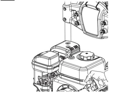
6 Allow engine to run for several seconds, then move choke lever to RUN position (see page 10).
